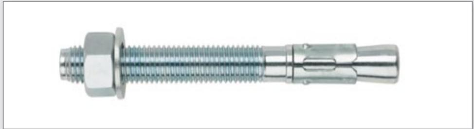
The recommended minimum diameter of the rod axis is 12 mm and it can be 14 or 16 mm in special cases. The minimum length required for anchoring in concrete should be 10 cm (5 cm within + 5 cm piece under floor) depending on the type and pavement condition. In any case, it is recommended to always consult the manufacturer's data sheet.
